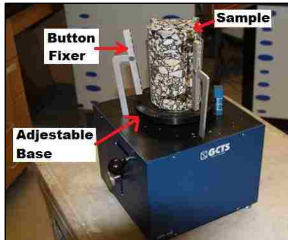
Figure 3.6: Automatic Positioning Fixture
